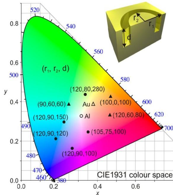
Fig. 4. Metallic color palette<sup>†</sup>: CIE1931 chromaticity diagram overlaid with points corresponding to the simulated reflected colors of single ring intaglio metamaterial designs in aluminum (circular symbols) and gold (triangles), labeled according to their structural parameters (external radius  $r_1$ , internal radius  $r_2$ , depth  $d$ , array period = 300 nm in all cases). Points for the unstructured metals are indicated by open symbols.
