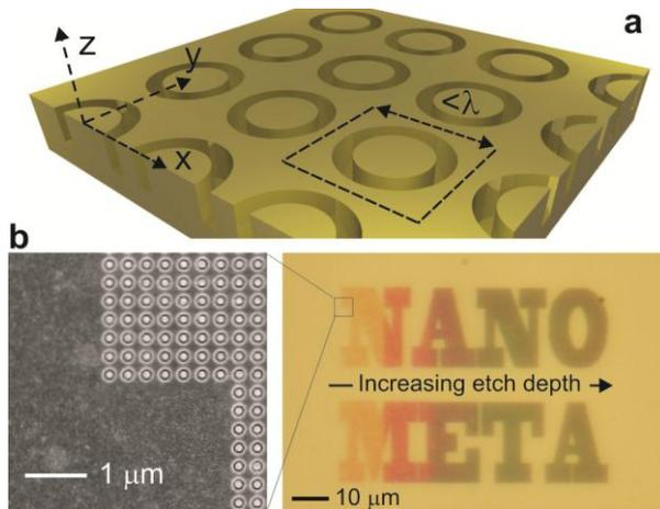
Fig. 1. Metallic structural color<sup>†</sup>: (a) Artistic impression of a generic intaglio metamaterial array of sub-wavelength single ring meta-molecules inscribed into a metal surface; (b) The realization of this concept in gold: The words 'NANO META' seen under an optical microscope on the right are formed from arrays of 170 nm diameter rings (as shown in the electron microscope image, left) milled to a depth that increases in six steps from 60 to 200 nm across the sample.
