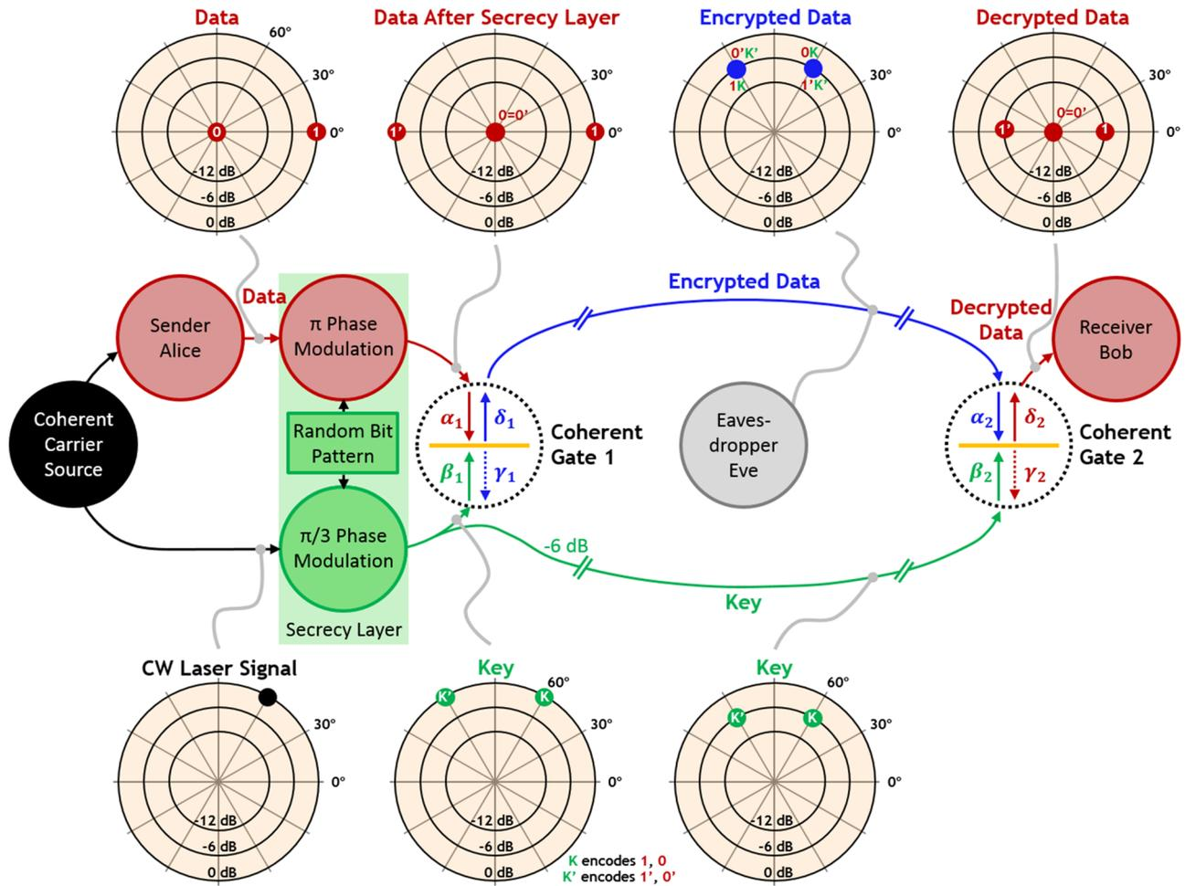
**FIG. 5.** Secure coherent encryption and decryption with secrecy layer. A secure encryption scheme, where neither the transmitted key nor the transmitted encrypted data alone reveals any information about the secret data. The binary logical states are represented by 0 and 1 and the key is represented by K, where ' represents a phase shift that is applied simultaneously to data and key for randomly chosen bits.
