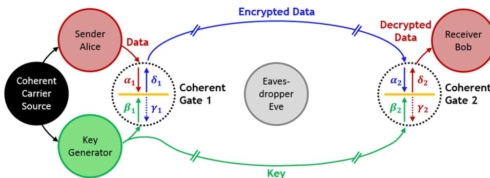
**FIG. 1.** Coherent encrypted information network. Alice encrypts her data by forming a coherent superposition of data and key on Coherent Gate 1. Bob decrypts the data by combining the encrypted data and the key on Coherent Gate 2. To eavesdrop the communication line, Eve would have the difficult task of detecting not only the intensity of the encrypted data and key signals, but also their mutual phase and shall also know the type of gate that has been used for encryption and decryption.
