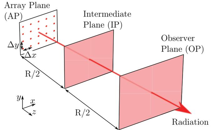
FIG. 7. (Color online) The (emitter) array plane, intermediate plane, and the observer plane used in the proof of validity of Eq. (5). The distances between the neighboring planes are  $R/2$  and the lengths of the rectangular unit cells of the array are  $\Delta x$  and  $\Delta y$ .
