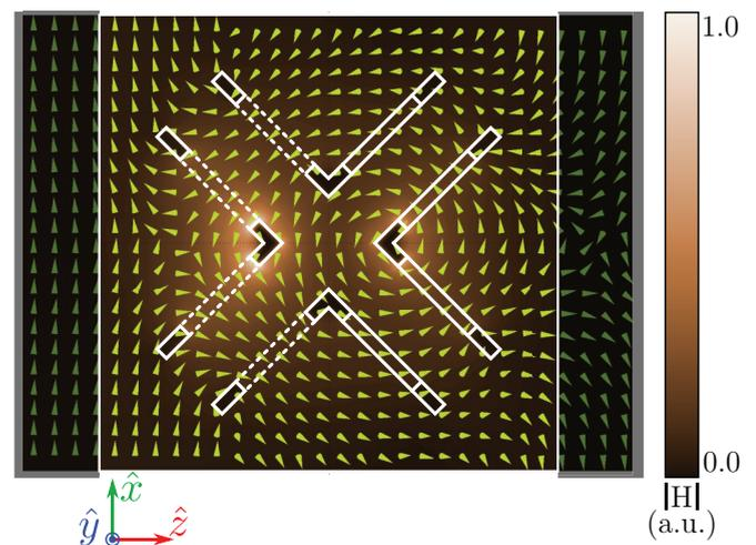
FIG. 10. (Color online) Distribution of magnetic field around the test-case metamolecule at the resonance ( $\lambda = 17.4 \mu\text{m}$ ). The arrow plot shows the direction of magnetic field while the color map on the background shows the magnitude of the field. The regions outside the metamolecule have been partially screened to highlight the unit-cell boundaries.
