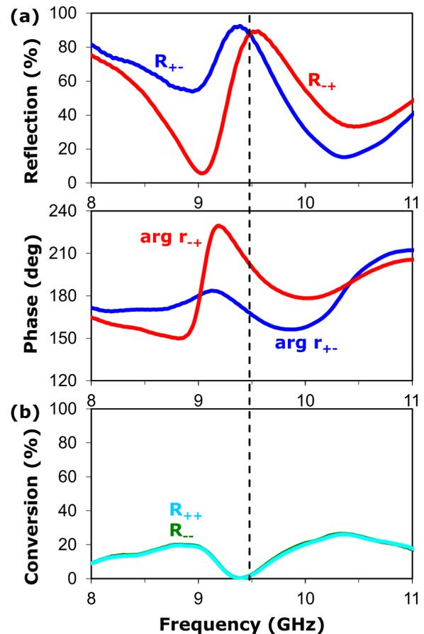
FIG. 2. Reflection spectra for both circular polarizations for the incidence angle of  $\alpha = +30^\circ$ . The dashed line indicates a frequency where both linear birefringence/dichroism and specular circular dichroism vanish.
