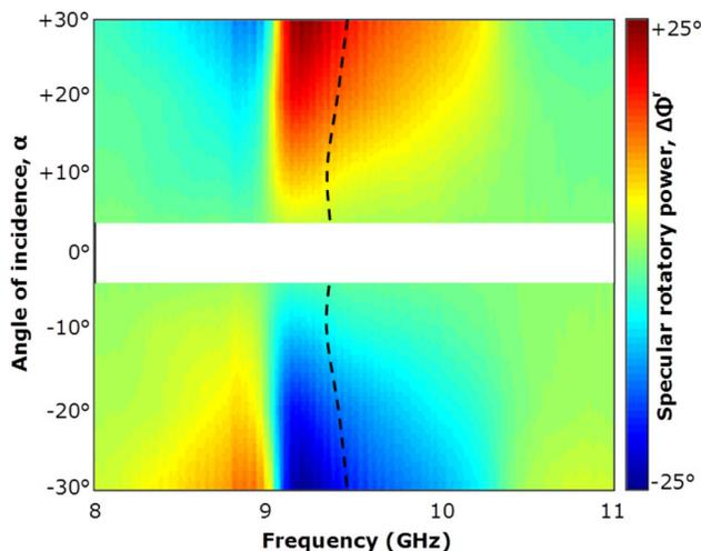
FIG. 4. Specular rotatory power in terms of azimuth rotation  $\Delta\Phi'$  for reflected linearly polarized waves as a function of the angle of incidence  $\alpha$  defined in Fig. 1(b). Simultaneous absence of specular circular dichroism and linear birefringence/dichroism is indicated by a dashed line.
