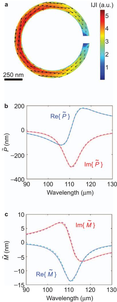
**Figure 2** (a) The on-resonance induced current in a GSR under the conditions described in Figure 1b. (b, c) The electric ( $\tilde{P}$ ) and magnetic ( $\tilde{M}$ ) polarizability densities: full simulation (solid curves) compared with the analytical expressions of Equation (5) for the parameters listed in the first row of Table 1. GSR, graphene split-ring.
