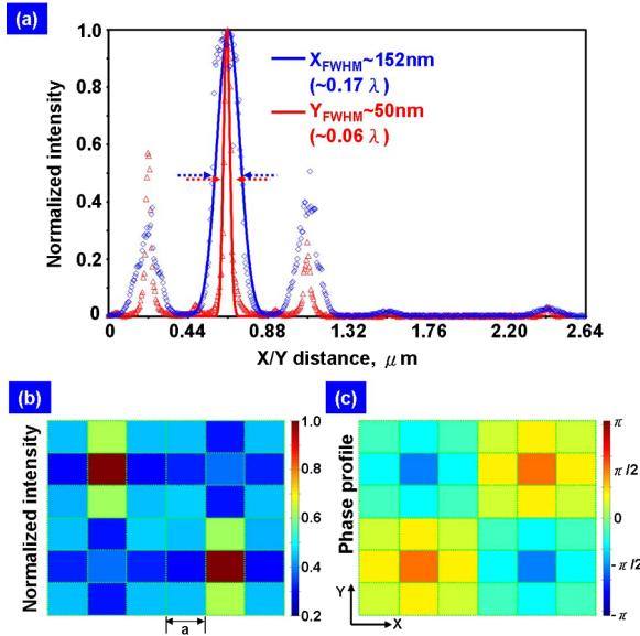
FIG. 3 (color online). The main cross sections of the energy hot spot (a) created at the metamaterial landscape corresponding to the conditions of Fig. 2(c) indicate a subwavelength localization with a footprint at the peak of about 1% of  $\lambda^2$  while there is no excitation on the other quadrant. Color maps (b) and (c) show the intensity and phase of excitations within the model of individual interacting dipoles representing the metamolecules of array.
