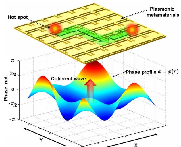
FIG. 1 (color online). Coherent control of light localization in an array of interacting metamolecules: artistic impression. A light beam with modulated phase profile excites a metamaterial array of interacting plasmonic resonators leading to the formation of the energy hot spot at the metamaterial. This spot may be moved from a metamaterial cell to another metamaterial cell by tailoring the phase profile of the incident beam.
