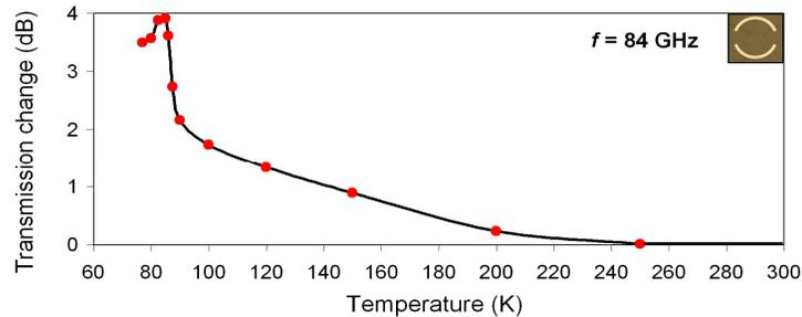
Fig. 3. Change of transmission measured at 84 GHz as a function of temperature for negative superconducting YBCO metamaterial (relative to its room temperature state). Experimental data is presented by red dots, while black curve provides guide for eye.
